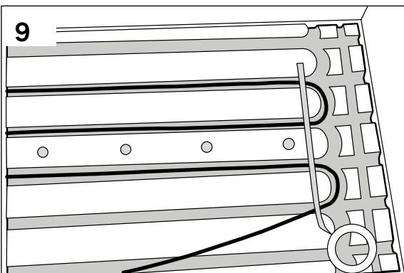
(Figure 10) If there is any excess cable when all grooves are filled, run it along the empty outer grooves, in the one close the outer walls in the first place.
