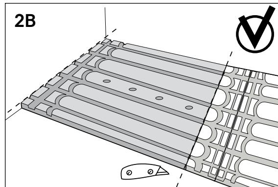
(Figure 3) Cut out a channel for the flexible floor conduit connected to the sensor for the floor heating thermostat. Then cut out a 10x30 cm square that is only 1 cm deep. The sensor will be placed here.
