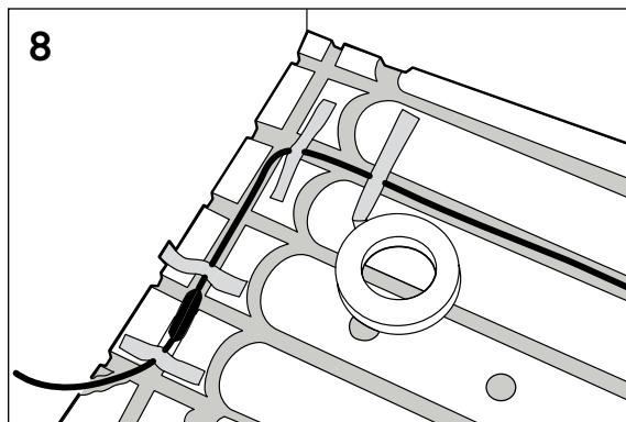
(Figure 9) Loop the cable back along the next outermost, wide groove. Tape directly inside the wide groove and leave the tape roll in place. Continue in this way until all the cable is drawn and all grooves, except the outer ones, are filled.
