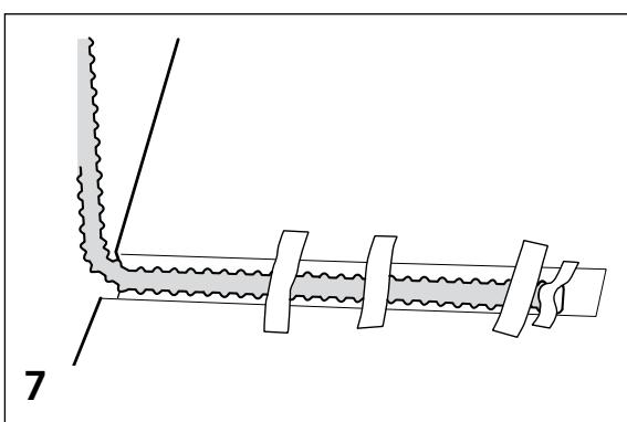
(Figure 4) Remove the boards. Prime the floor and allow it to dry. Apply the adhesive using an 8-10 mm serrated spreader.
