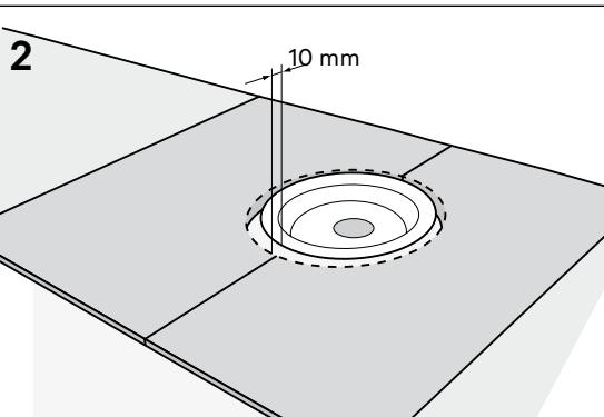
(Figure 3) Cut out a channel for the flexible floor conduit connected to the sensor for the floor heating thermostat. Cut entirely through the board and at the same width as the conduit.
